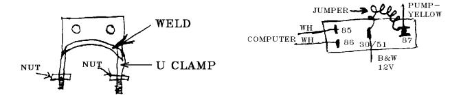
E-ES FUEL PUMP RELAY: When these fail, the fuel pump won't run. This relay is 2nd from the firewall on the passenger side. In an emergency, it can be bypassed as follows: Run a jumper wire from the center terminal (#30/51- hot) to the yellow wire (#87). The pump will turn on with the ignition switch. You can probably drive this way indefinitely.
